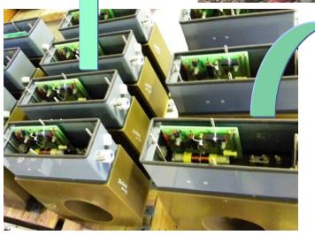
Voltage Limiter & Filter Capacitors in option
